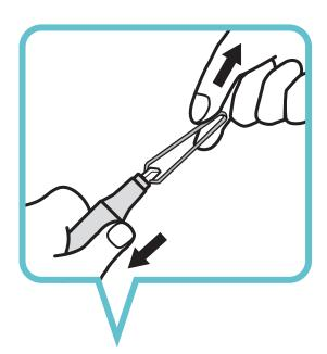
Using the tweezers, pull the large nib out of the marker. Insert the new nib slowly back into the marker. The ink will wick from the inside out to the end of the nib. This may take a few minutes.
